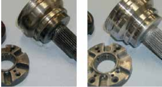
Removal of oxidation and other contaminants
